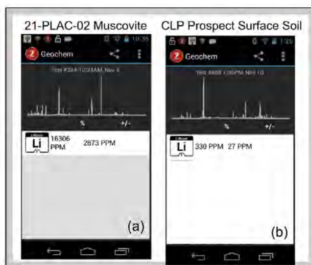
Figure 13. Screen shots from the Z-300 Geochem mode for a muscovite from Carolina Lithium Project prospect pegmatite outcrop sample 21-PLAC-02 (a) and a surface exposure of the Cecil soil on the CLP prospect (b). The Z-300 screenshots show the broadband LIBS spectrum recorded for each sample and estimated elemental abundances derived from the spectral emission line intensities. The Li content for the muscovite was determined from the mica calibration of Figure 11, whereas that for the Cecil soil was determined from the pegmatite powder calibration of Figure 12.
