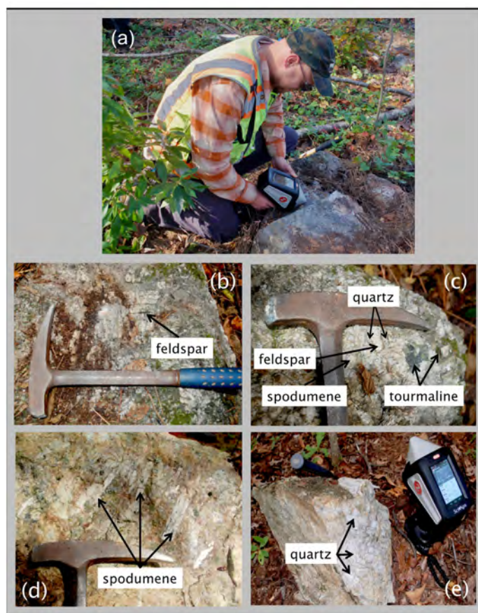
Figure 4. In-field LIBS analysis of pegmatite outcrops on the Carolina Lithium Project prospect in Gaston County, N.C., showing the use of the handheld LIBS analyzer for in-situ analysis (a) and examples of the different minerals analyzed—feldspar (b); feldspar, quartz, spodumene, and tourmaline (c); spodumene (d); and quartz (e).
